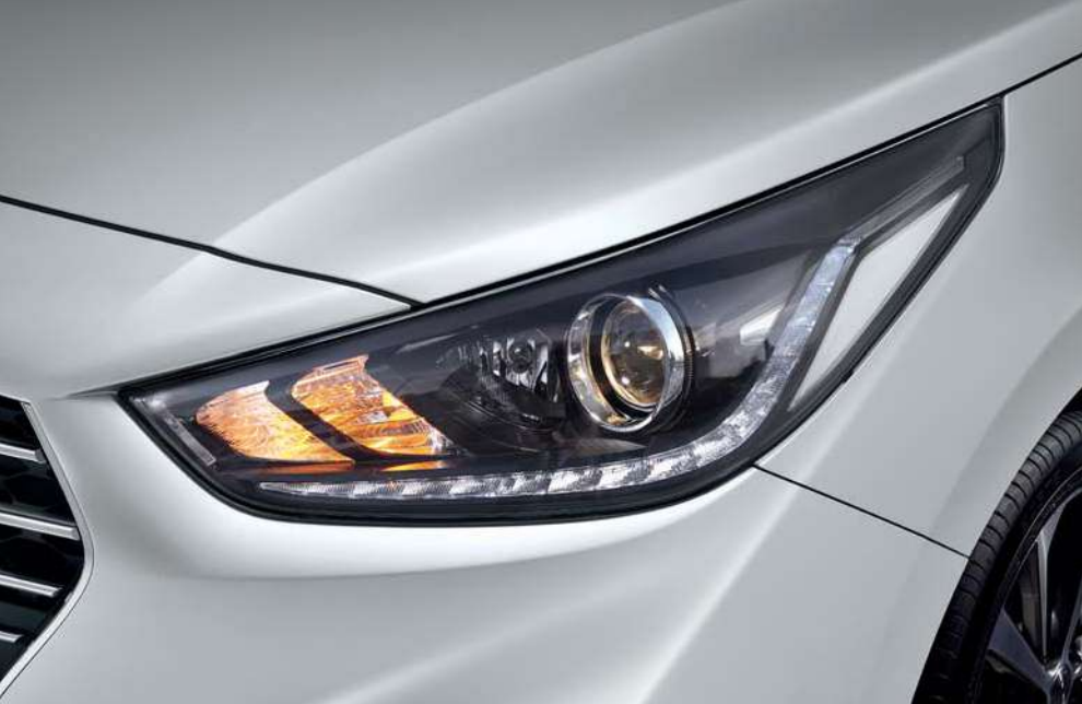
Projection headlamps with LED position & DRL lamps
