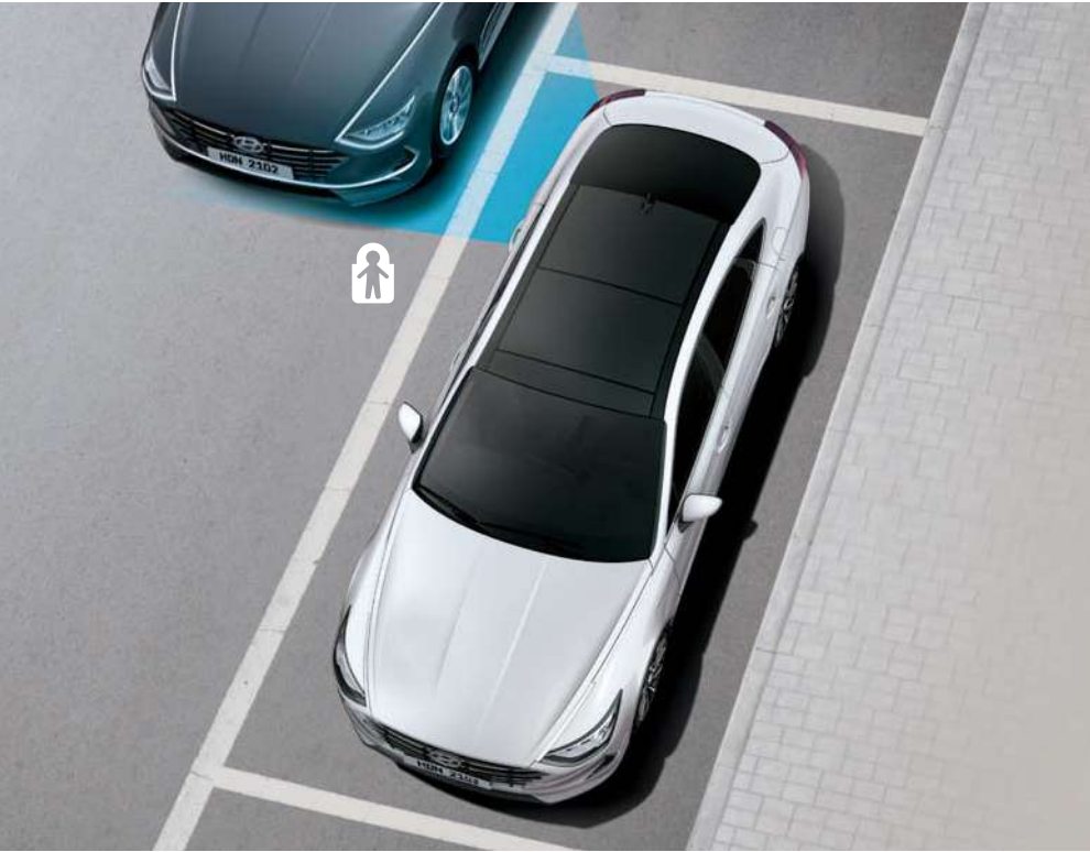
Safe Exit Assist (SEA) SEA blocks any attempt to disengage the child safety lock and prevents the rear door from opening when it is unsafe to do so. On detecting the presence of a rear seat passenger and the approach of a vehicle from the rear, SEA will also flash a pop-up message on the cluster and will issue an audible alarm, alerting the driver to the danger.
