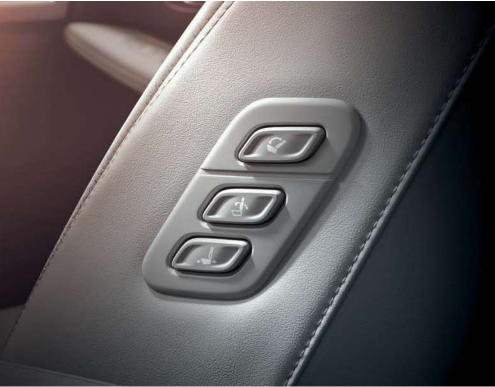
Walk-In device The walk-in device button extends front seat control functions to the rear seat passenger such as chauffeured executives who may want extra legroom. It's one of many interior details that demonstrate careful consideration for comfort and convenience.
