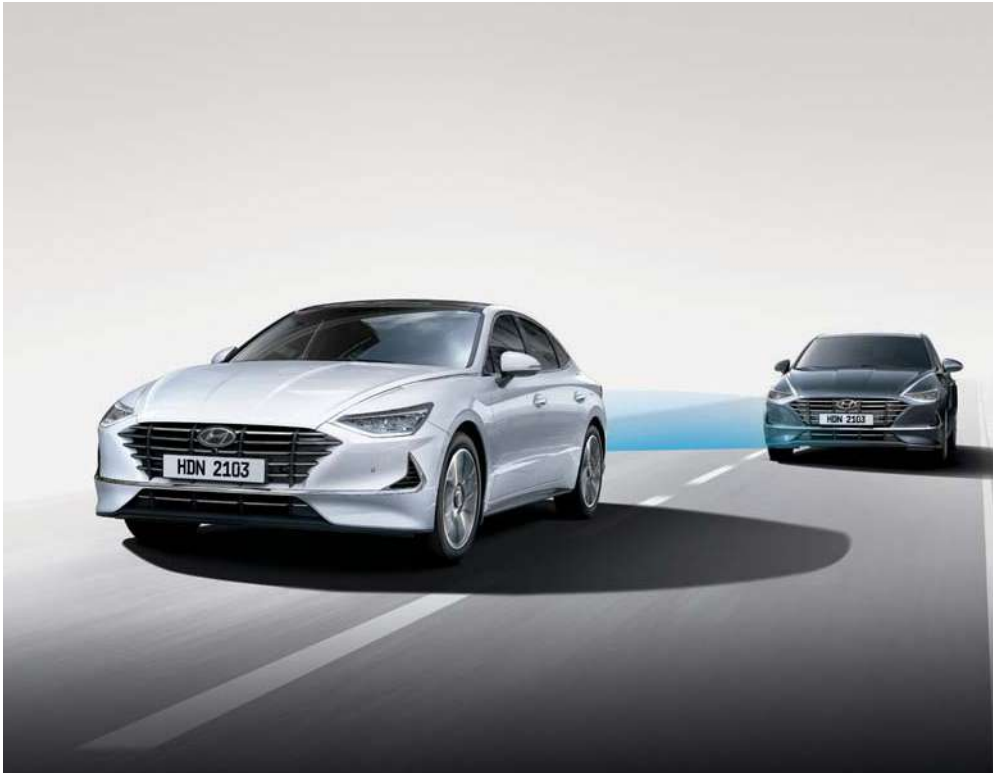
Blind-spot Collision Warning (BCW) BCW provides visual and audible warnings when there is an object in a blind spot while changing lanes.
