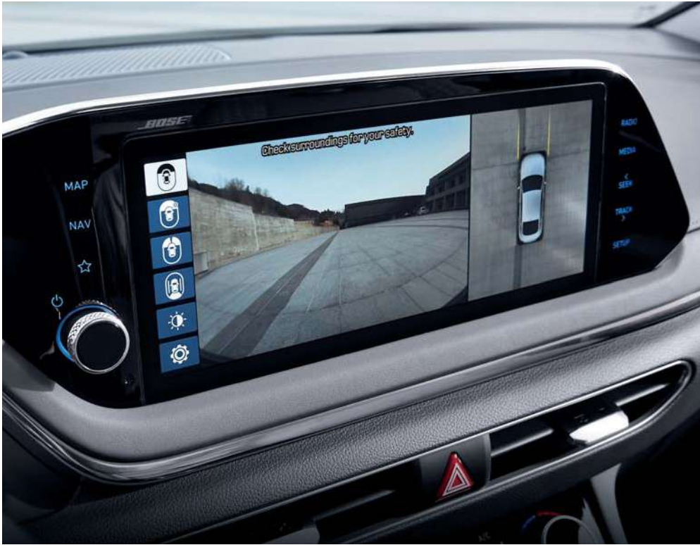
Surround View Monitor (SVM) SVM uses the AVN head unit to serve up a 360-degree birds eye view of the car and its surroundings. This optional system comes in quite handy when trying to fit the car into a tight parking spot.
