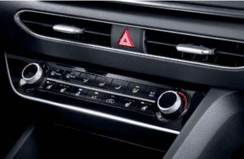
Manual air conditioning system
